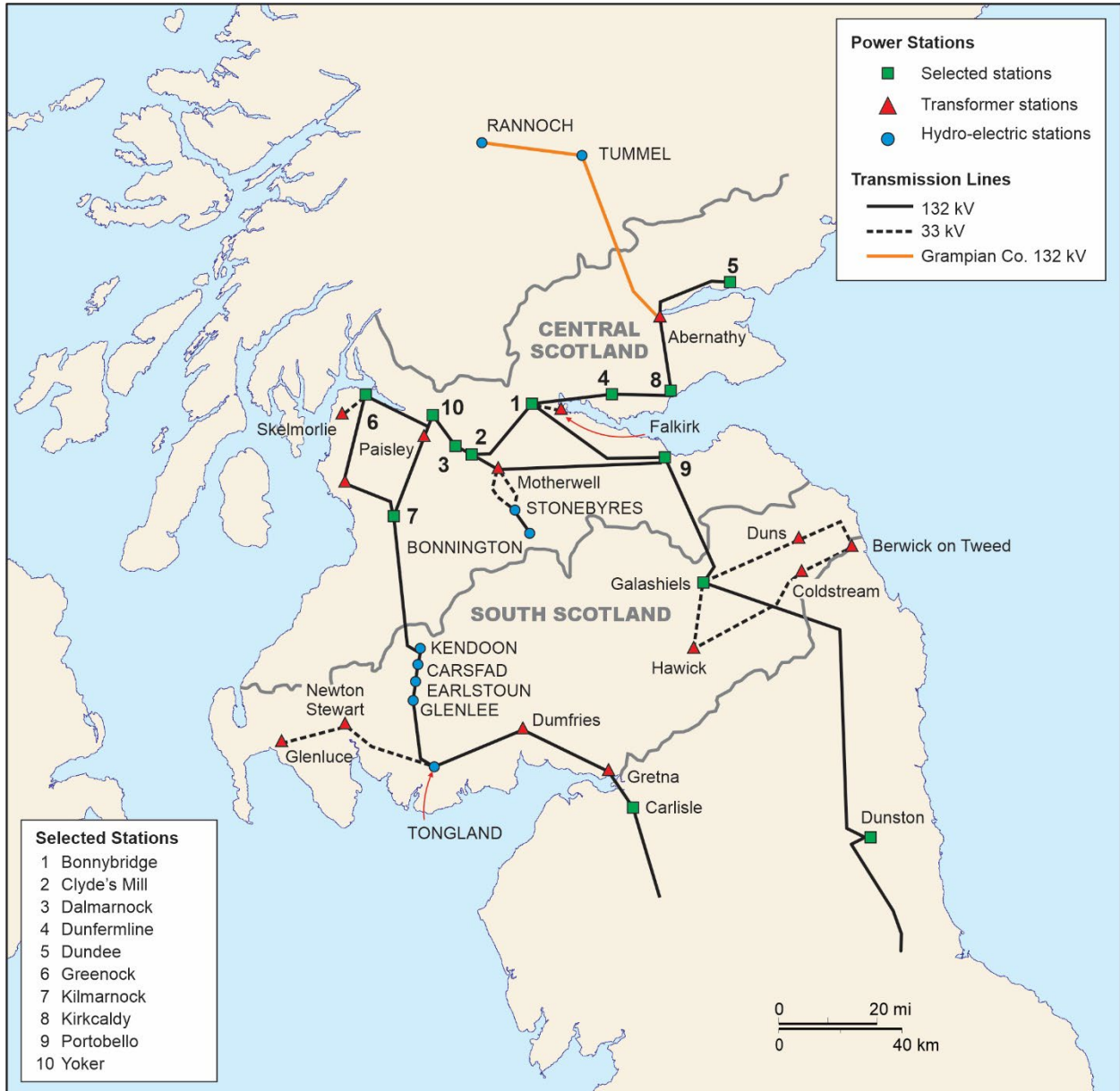
Figure 4 CENTRAL AND SOUTH SCOTLAND ELECTRICITY SCHEMES 1936.
